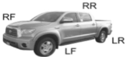
Prefit and ensure both driver side and passenger side fender flares to the vehicle before painting or installation. You may remove any moldings, strips or existing flares from the vehicle for fitting or installation. You can cut the fender flare to fit any body side molding.
