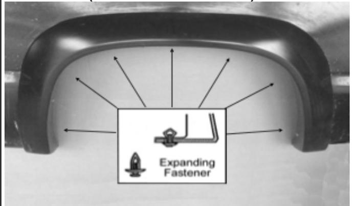
Place the flare on the vehicle. Apply 7 Plastic Expanding Fastener into the mounting slots in flare and secure it to the vehicle as shown.
