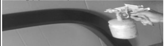
Professional painter or body shop recommended to paint flares. Follow all the paint manufacture specifications to paint the flares. Clean fender flare surfaces with clean water and a mild detergent before painting, do not use lacquer thinner or any solvent based products.
