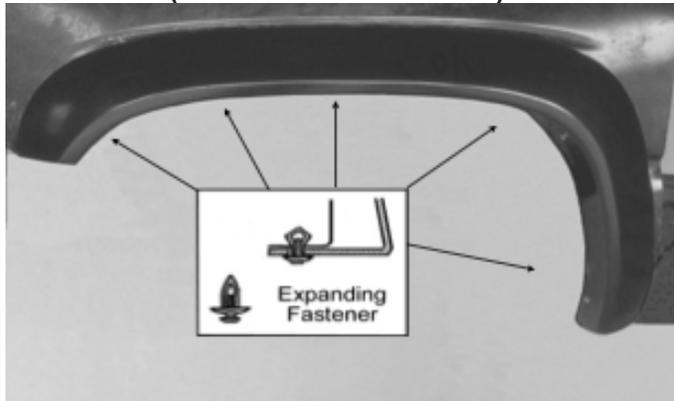
Place the flare on the vehicle. Apply 5 Plastic Expanding Fasteners into the mounting slots in the flare and secure it to the vehicle as shown.
