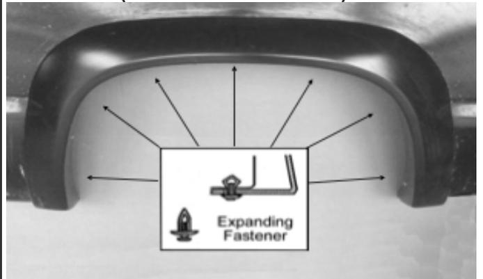
Place the flare on the vehicle. Apply 7 Plastic Expanding Fasteners into the mounting slots in the flare and secure it to the vehicle as shown.
