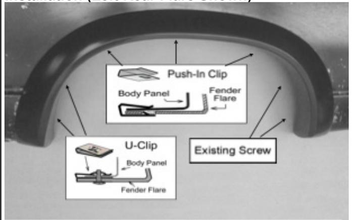
Place the flare on the vehicle. Apply 3 Push-In Clips into the mounting slots in the flare and secure it to the vehicle, 4 U-Clips secure into the hole with screws as shown. Fasten the existing factory screws into the original location that were previously removed.
