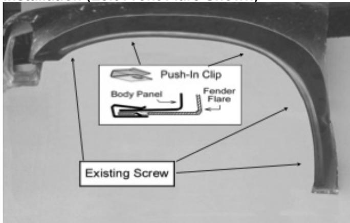
Place the flare on the vehicle. Apply 2 Push-In Clips into the mounting slots in the flare and secure it to the vehicle as shown. Fasten the existing factory screws into the original location that were previously removed.
