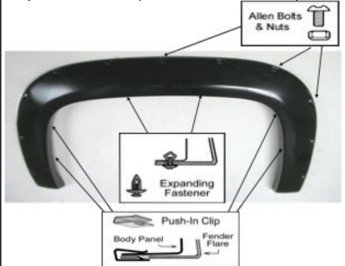
Place the flare on the vehicle. Apply 5 Push-In Clips into the mounting slots in the flare and secure it to the vehicle as shown.
