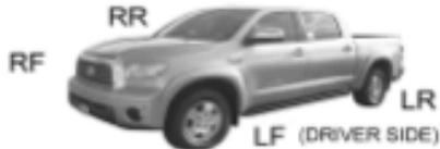
Pre-fit both driver side and passenger side fender flares to the vehicle before painting or installation. You may remove any moldings, strips or existing flares from the vehicle for fitting or installation. You can cut the fender flare to fit any body side molding.
