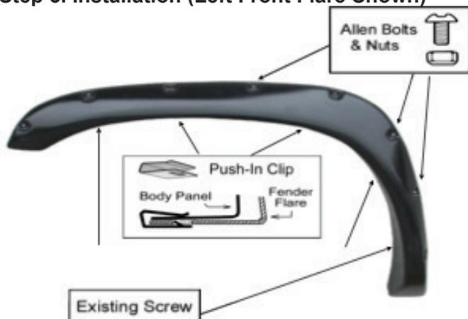
Use torx bit to tighten allen bolt & put firmly on every pocket of the fender flares first. Place the flare on the vehicle. Apply 2 Push-In Clips into the mounting slots in the flare and secure it to the vehicle as shown. Fasten the existing factory screws into the original location that were previously removed.
