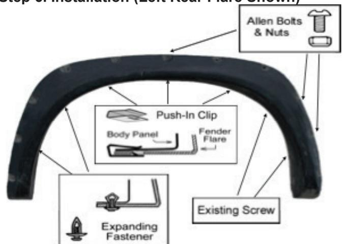
Use torx bit to tighten allen bolt & put firmly on every pocket of the fender flares first. Place the flare on the vehicle. Apply 3 Push-In Clips into the mounting slots in the flare and secure it to the vehicle. Apply 2 Plastic Expanding Fasteners into the mounting slots in the flare and secure it to the vehicle as shown. Fasten the existing factory screws into the original location what were previously removed.
