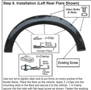
factory screws into the original location that were previously removed.
