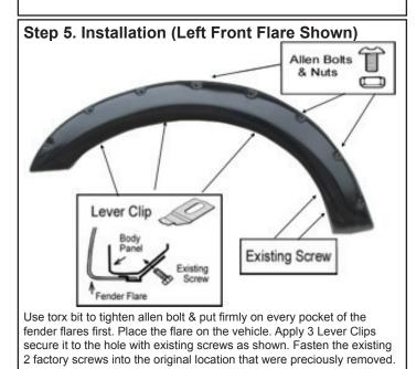
Qty (2) U-Clamp with Flat Head Screws Qty (6) J-Clips Qty (6) Lever Clips Qty (36) Allen Bolt & Nut (Torx Bit required) Qty (8) Self Tapping Screws (see option B)
