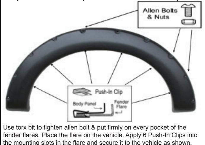
Use torx bit to tighten allen bolt & put firmly on every pocket of the fender flares. Place the flare on the vehicle. Apply 6 Push-In Clips into the mounting slots in the flare and secure it to the vehicle as shown.
