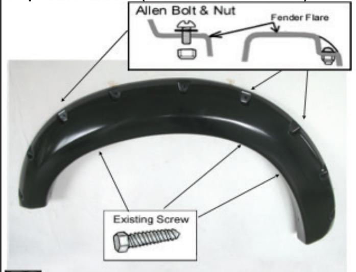
Use torx bit to tighten allen bolt & put firmly on every pocket of the fender flares. Place the flare on the vehicle. Apply 5 Push-In Clips into the mounting slot in the flares and secure it to the vehicle as shown.
