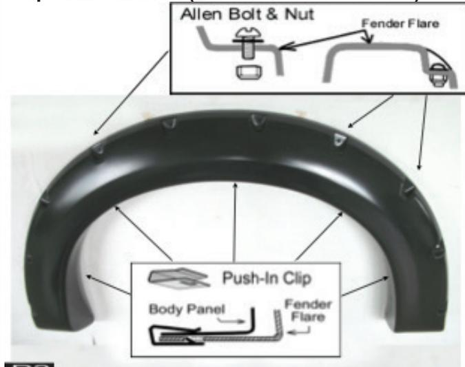
Use torx bit to tighten allen bolt & put firmly on every pocket of the fender flares. Place the flare on the vehicle. Fasten the existing factory screws into the original location that were previously removed.
