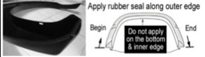
Apply rubber seal to the flare. Start at one end of the flare along the edge that comes in contact with the body panel. Apply pressure on the tape to ensure adhesion, and trim excess rubber seal at the end. To avoid bulge, you may cut a notch in the edge of the rubber seal at the inward angle curve, cut a V out of the outward angle curve.
