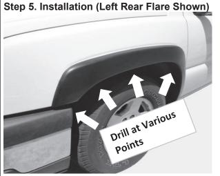
Using a 1/8" diameter drill bit or the provided self tapping screws, attach the flare at the various points.
