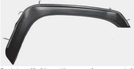
Peel about 2" of the red liner away from one end of the double sided adhesive tape. Pulling the red liner free attach the flare to the fender with firm and even pressure to ensure adhesion.
